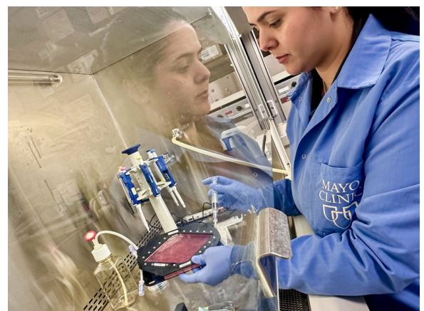
NASA Image: JSC2026E014320 - The BioServe stem cell bioreactor is being prepared for a preflight test run by Mayo Clinic researcher Fay Ghani as part of InSPA-StemCellEX-H2. This investigation works upon prior research to produce stem cells in greater numbers in a space environment with BioServe's newly developed microgravity bioreactor. Credit: Mayo Clinic.
